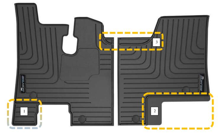
Trims for the front driver and passenger side liners are highlighted above. These trims accommodate fire extinguisher positions on the driver's side and seat base variations on the passenger side. At the top of the parts, there is a possible trim that accommodates dash base shapes. When trimming, leave the protective rib wall on the liner (see images of trim in image below).
