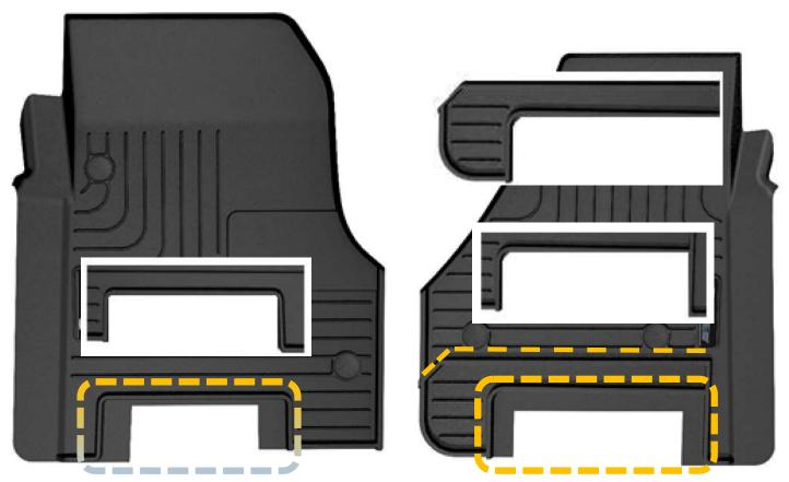
Trims for the front driver and passenger side liners are highlighted above. These trims accommodate seat variations available in Freightliner Cascadia models. When trimming, leave the protective rib wall (see images of trim in insert images). The passenger side liner has a larger trim for models with the battery box under the passenger side seat.
