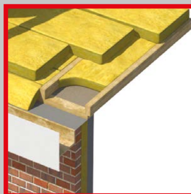
Lofts - Insulating between and over joists
