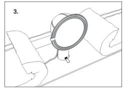
If you prefer to have your Thermahood adhered to the ceiling, take the cover off and apply water based adhesive around the rim of the hood or use Air-tightness tapes and/or adhesive.
