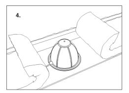
Thermahood can now be fitted to the ceiling lining. Make sure to keep enough slack on wires in order to change the bulb/lamp.
