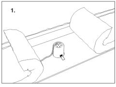
Clear the area around the downlight and clean dust from ceiling lining (plasterboard etc.)
