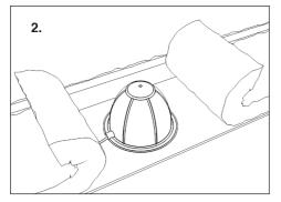
Place Thermahood over the downlight, bring the wire through the aperture on the rim of the cover; a double wire should also fit neatly into the aperture.
