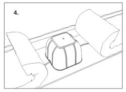
Thermahood can now be fitted to the ceiling lining. Make sure to keep enough slack on wires in order to change the bulb/lamp.
