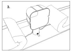
If you prefer to have your Thermahood adhered to the ceiling, take the cover off and apply water based adhesive around the rim of the hood or use Air-tightness tapes and/or adhesive.
