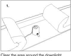
Clear the area around the downlight and clean dust from ceiling lining (plasterboard etc.)
