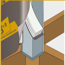
Separate the insulation layers and cut them away to leave the membrane layer only in the valley gutter.
