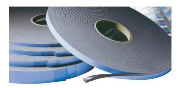
Double Sided high tack acrylic adhesive coated PVC structural spacer glazing tape. This tape is designed for use in structural spacer systems and has an open cell structure to allow the curing of structural silicones on all sides. Fast recovery from compression.
