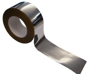
Novia Metallised BOPP (Biaxially Oriented Polypropylene) tape is an extremely high tack, high tear resistant, low emissivity and low moisture vapour permeability lap sealing tape for use in all air and vapour control layer and damp proof membrane applications.
