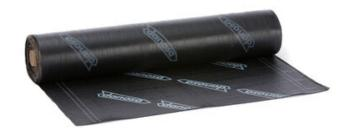
GLASDAN 30 P POL is a waterproofing bituminous sheet with non self-protected surface of 3.0 kg/m². Composed of a fibreglass reinforcement and covered on both sides with polymer modified bitumen mastic. A polyethylene film is used as anti-adherent material on both sides. Tested according to standard EN test methods.
