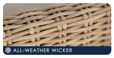
We manufacture all-weather wicker from the highest quality man-made HDPE fibre. This remarkable material has many benefits including high suppleness, tear resistance, UV resistance and weather resistance.
