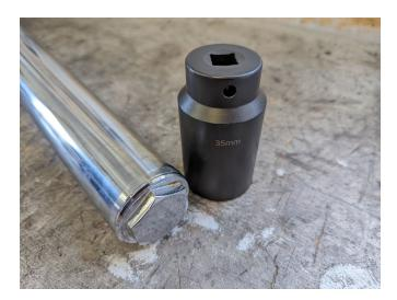
• TC Tip: By following this sequence of steps, loosening the fork caps is made easier because the fork tubes remain stationary. A 35mm socket is required to remove most factory fork caps.
