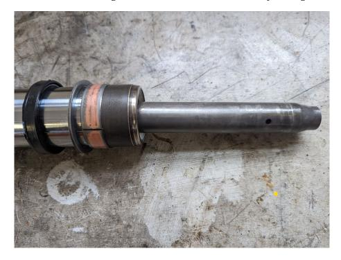
Install new damper rod bolts and new damper rod crush washers to factory torque specification.
