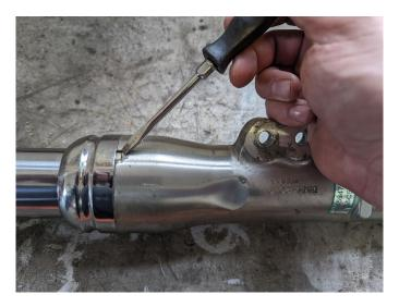
Free the seal retaining rings from their grooves in the lower leg.
