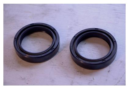
Install new sealing rings on the damper rods.
