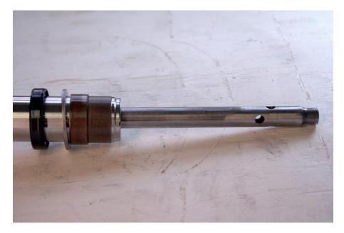
Install new damper rod bolts and new damper rod crush washers to factory torque specification.
