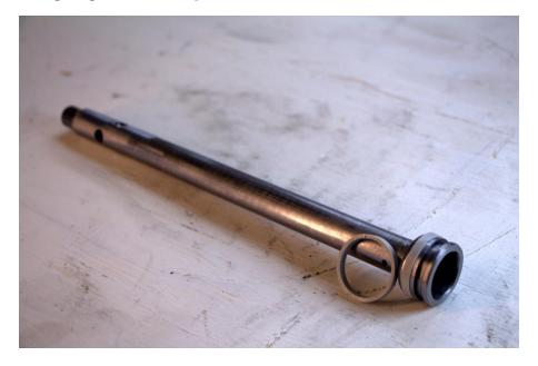
Install rebound springs onto damper rods. Insert damper assemblies into fork tubes. Return damper rod bases to the lower legs. Slide each tube into its corresponding lower leg.
