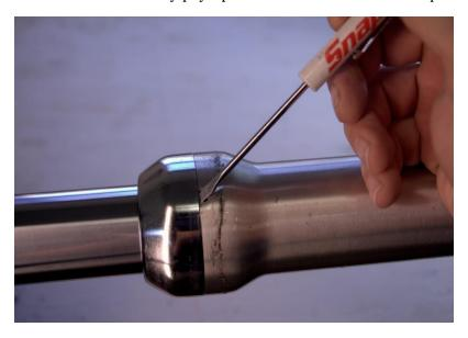
Free the seal retaining rings from their grooves in the lower leg.
