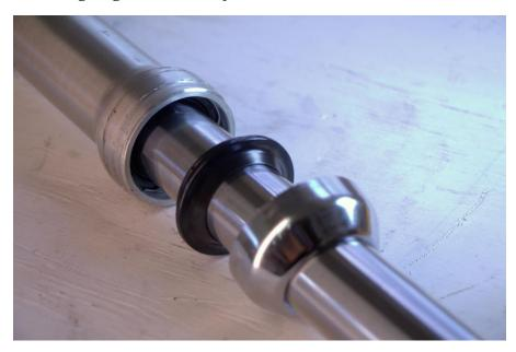
Install fork tubes into the triple trees. Be sure fork tube protrudes slightly above the top tree. Tighten to recommended torque specification. Extend the tubes fully.
