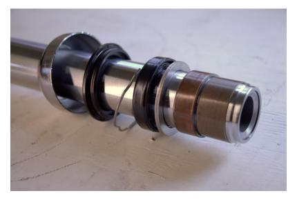
Measure correct fluid quantity, and pour into the fork tubes. Check for leaks at the damper rod bolt. If leaks are found, re-check torque at bolts, drain tubes, and fill again with the correct quantity of fluid.
