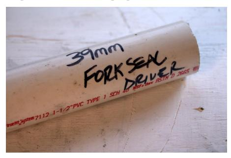
Reinstall seal retaining rings, new seal wipers, and dust boots.
