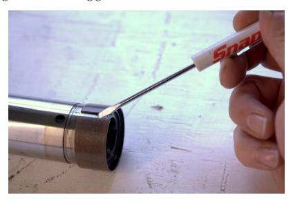
Install slider bushings (the upper bushing when fork is upright) and backup rings onto fork tubes from the top.
