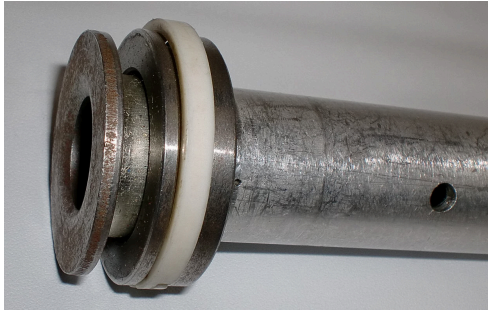
Flat-Top Suzuki DR350 Emulator Adapter Built into Emulator FEGV 4321
