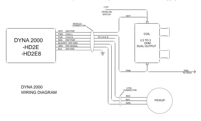
\*\*NOTE\*\* RECOMMENDED COIL: USE ONE DUAL OUTPUT COIL WITH 2.5 TO 3 OHMS PRIMARY RESISTANCE, SUCH AS DYNATEK PART NO. DC6-1 OR DYNATEK PART NO. DC1-1.
