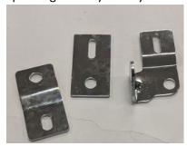
7. Loosely install bottom exhaust pipe to rear & middle mounting brackets. Do not tighten bolts.
