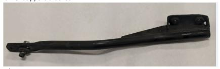
4. Locate hardware pack/mounting brackets included with the new exhaust
