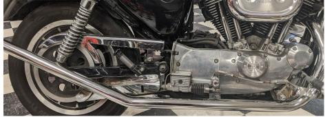
8. Loosely install top exhaust pipe to rear slotted mounting bracket on bottom exhaust pipe. Do not tighten bolts.
