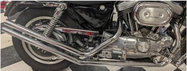
10. Begin by tightening the top and bottom exhaust pipes together in the rear (while holding them parallel), tighten the rear bracket to the bottom pipe, then tighten the rear exhaust bracket (two larger bolts) to the frame of your sportster. Next tighten the mid (engine) mount to the bottom exhaust pipe. Finally, tighten your flange nuts to the head of your motorcycle.
