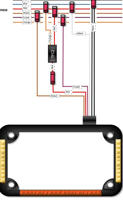
Diagram depicts the wiring color codes for a typical Harley-Davidson wire harness, when installing on other makes, please refer to your owners manual or service manual for the appropriate wire color codes. Use a meter and or test light to determine wire function if the former is not available. Not for use with bikes without a center tail light. If using with a Run Brake Turn Controller, the product must be installed before the RBT signal for correct operation.
