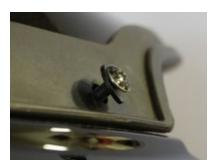
Ensure the washers on each mounting screw are out toward the head of the screws
