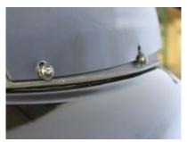
Install your new Flare™ Windshield onto the mounting screws. Torque the two center screws first, then the two outer screws.
