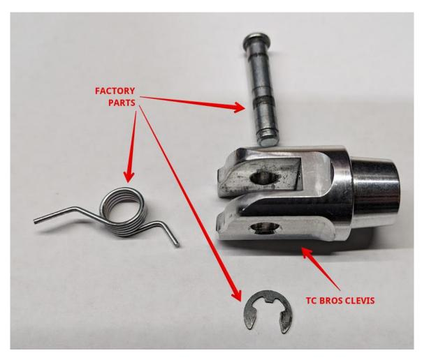
Factory hardware identified in picture. All factory pivot hardware will be reused.
