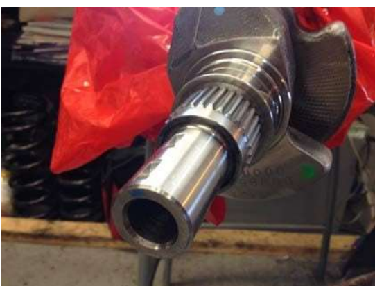
N1 collar and Inner gear
