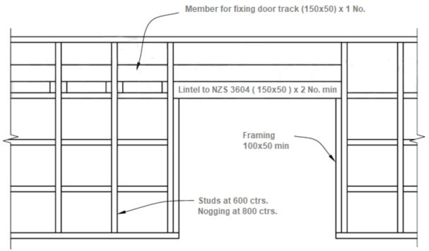
Elevation of typical framing at lintel
