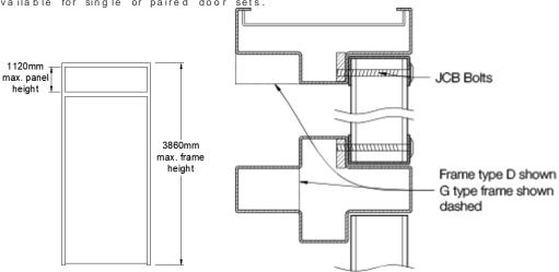
An overpanel without transom is available to an overall height of 3600mm with maximum door leaf dimensions 2400x1200, in single leaf only. The fire rating of this door set is -/90/60. Transomless overpanels are not available on this door type.
