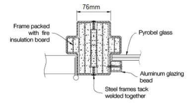
Note: Pyrobel glazing can be used for interior applications only.
