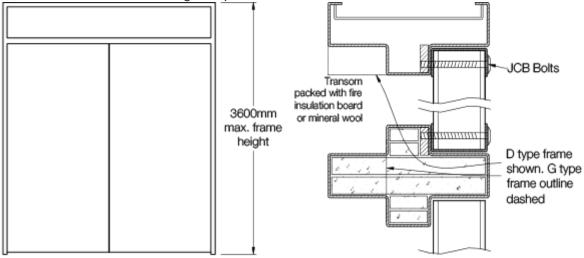
A complete door set with screw fixed side panels can be supplied, with the steel mullion between panel and door leaf to be grout-filled during installation.
