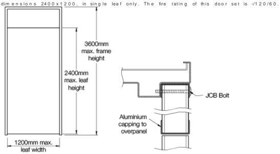
A complete door set with screw fixed side panels can be supplied, with the steel mullion between panel and door leaf to be grout-filled during installation.
