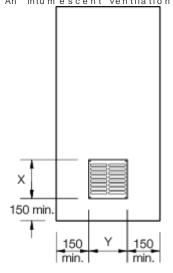
$\label{eq:decomposition} \mbox{Drop shutter grilles are not an option on this doorset.}$
