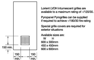
Please note that fire doors with ventilation grilles cannot be certified as 'Smoke' control door sets. Drop shutter grilles are not an option on this doorset.
