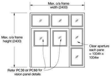
Alternatively a wall segment of minimum width 250mm must separate the FW60 fire window from a PC60 door set.
