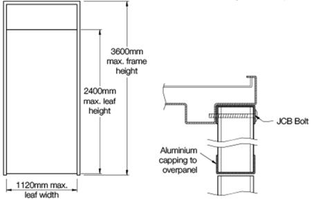
A complete door set with screw fixed side panels can be supplied, with the steel mullion between panel and door leaf to be grout-filled during installation.
