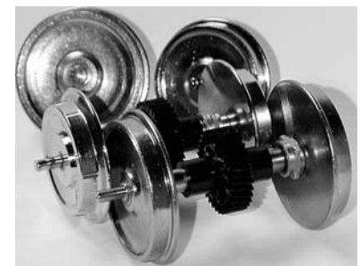
Left front—USA Trains 'toy flange' wheel; right front— NWSL #2521-6 36"/270 (Gear not included)
