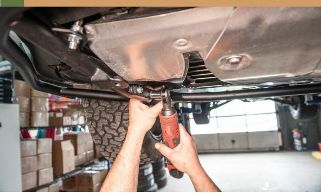
TIGHTEN SUPPORT ROD NUTS
