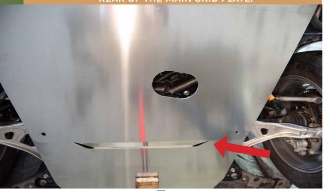
RE INSTALL THE SKID PLATE SPACERS.IF YOU DO NOT HAVE THE MAIN SKID YOU JUST NEED TO INSTALL THE SKID PLATE SPACERS
