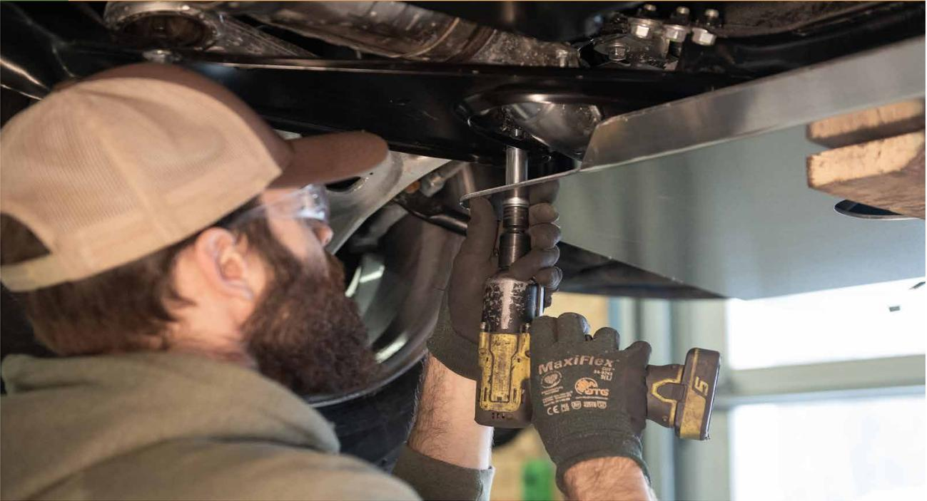
**2B** IF YOU DO NOT HAVE A MAIN SKID PLATE, REMOVE TWO BOLTS FROM FRONT A-ARM SUPPORTS
