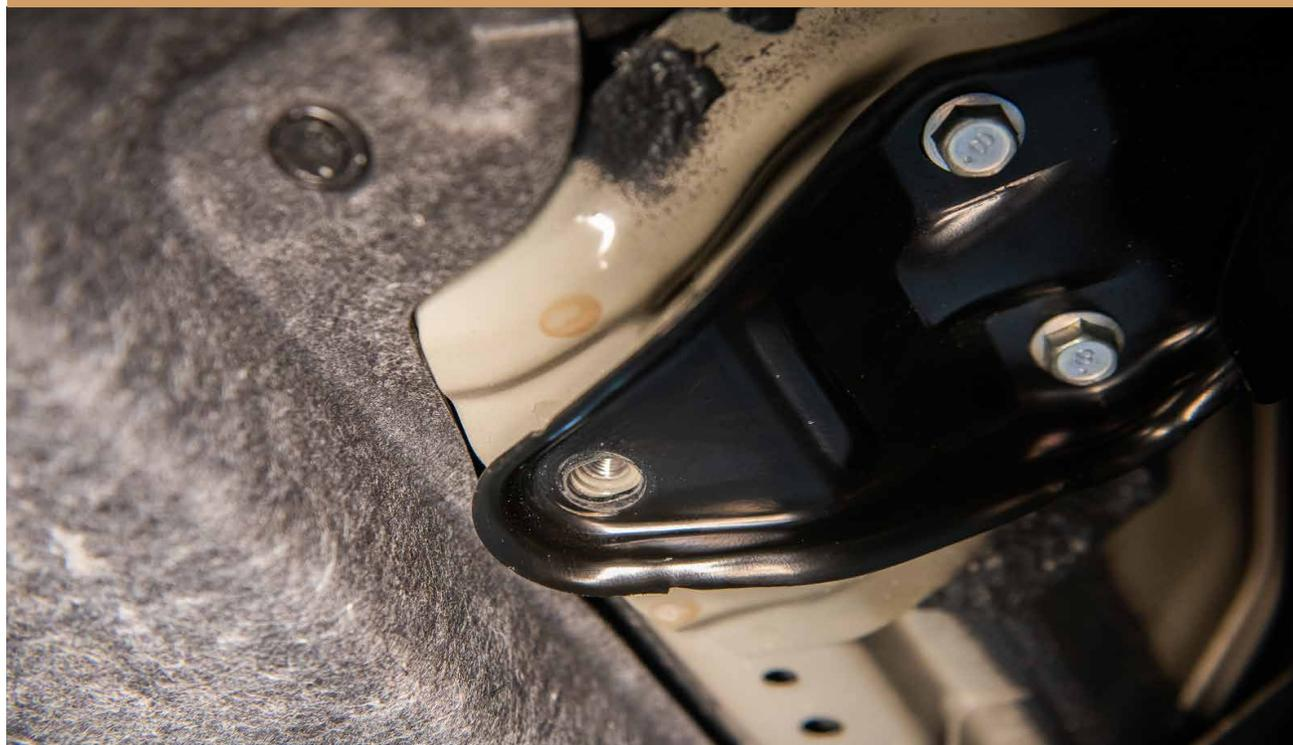
**2A** WITH A MAIN SKID PLATE, REMOVE REAR BOLTS AND SPACERS
