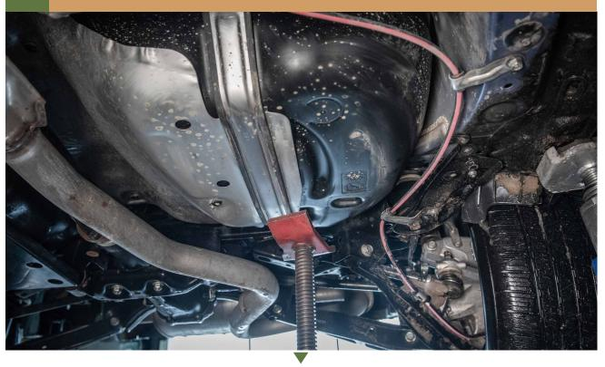
**9** USING THE CORRECT SKID PLATE SPACERS FOR YOUR APPLICATION AND THE SUPPLIED BOLT AND WASHER, INSTALL THE SKID PLATE INTO PLACE.
