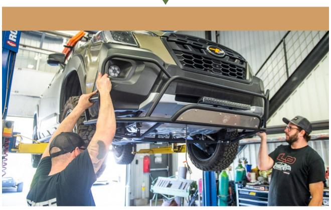
7 PLACE THE INCLUDED WASHER INBETWEEN THE BUMPER GUARD MOUNTING BRACKET AND THE VEHICLES LOWER TOW HOOK
