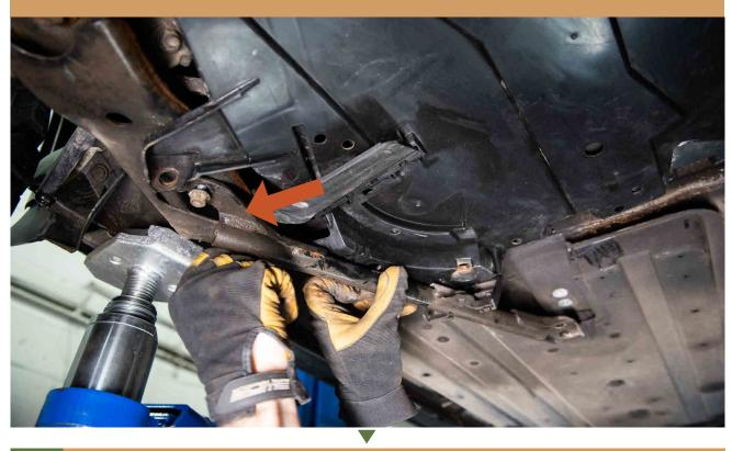
**INSTALL SUB FRAME SUPPORT BAR SPACERS**
