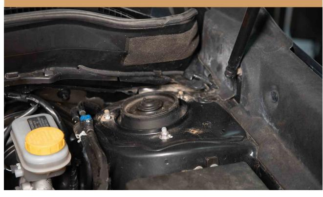
WHILE HOLDING THE STRUT ASSEMBLY 7 **REMOVE THE LAST STRUT NUT**
