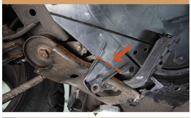
**RE INSTALL SUB FRAME SUPPORT BAR**
