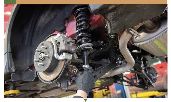
RE INSTALL LOWER BOLTS FOR SHOCKS AND KNUCKLES
