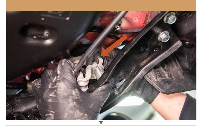
USE A SCREW DRIVER TO KEEP THE BRACKET FROM TURNING WHEN YOU TIGHTEN THE BOLT DOWN.
