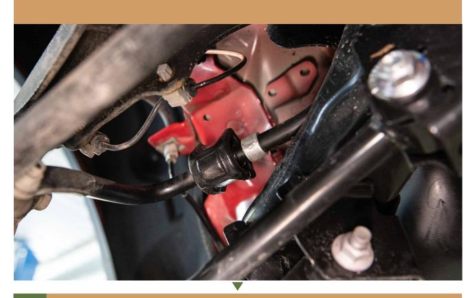
41 INSTALL THE SPACER FOR THE SWAY BAR MOUNT
