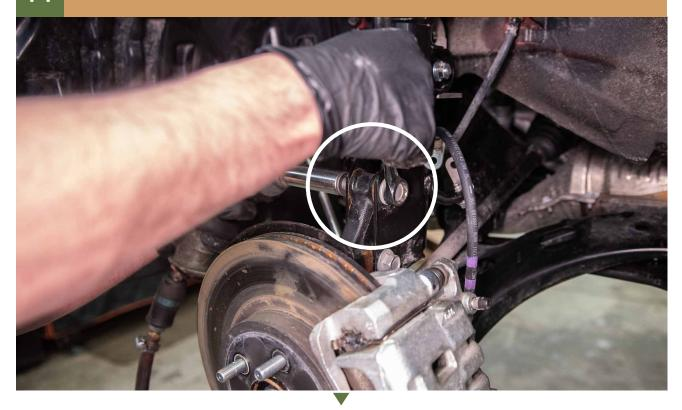
15 RE SECURE THE SWAY BAR LINK TO THE EXTENDED MOUNT
