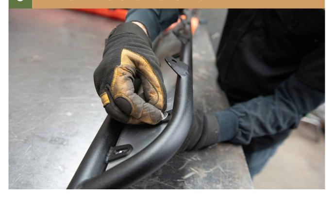
WITH THE TWO OUTER BOLTS HOLDING THE FRONT PLATE INPLACE, INSTALL THE REST OF THE NUTS AND BOLTS BUT DO NOT TIGHTEN YET.
