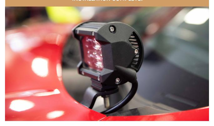
SPECIAL TIP: WHEN INSTALLING YOUR FOG LIGHTS ONTO YOUR NEW HOOD LIGHT BRACKETS. USE THE PROVIDED HOLES TO HELP SECURE THE CABLE
