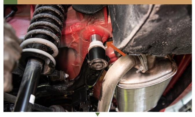
29 INSTALL THE SUPPLIED BOLTS WITH THE FACTORY PLATE INTO THE REAR OF THE SUB FRAME
