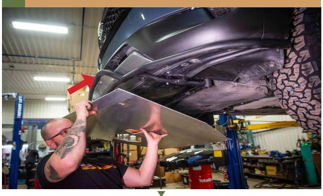
WHILE HOLDING THE SKID INPLACE, THREAD THE FRONT BOLTS IN. \*IF YOU HAVE THE OPTIONAL RALLY WASHERS, NOW IS THE TIME TO INSTALL
