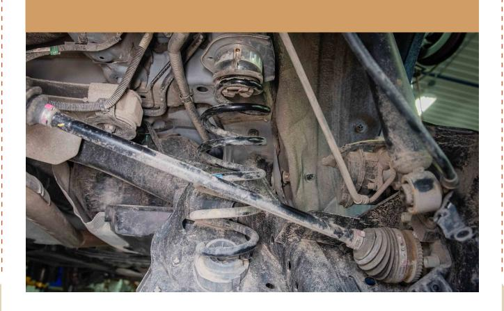
UN BOLT AND REMOVE THE SHOCK
