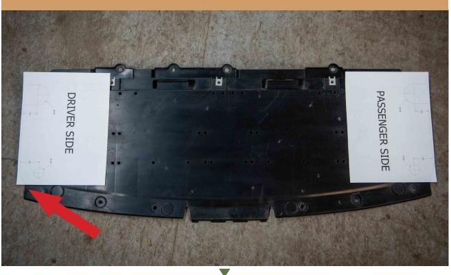
WITH THE TEMPLATES INPLACE, MARK THE CENTER OF THE HOLE. \*THE 2" HOLES NEED TO BE OPENED RIGHT TO THE EDGE USING A KNIFE
