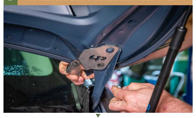
3 USE FACTORY BOLT TO SECURE HOOD LIGHT BRACKET, SNUG UP THE BOLT BUT DO NO FULLY TIGHTEN YET.
