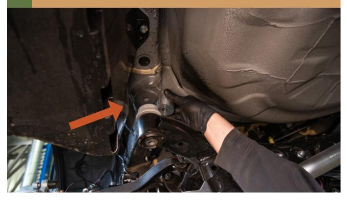
30 USING THE SUPPLIED BOLTS AND THE SUB FRAME WASHER PARTIALLY THREAD IN THE SUB FRAME
