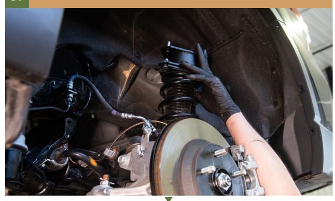
RE ATTACHE LOWER STRUT AND KNUCKLE BOLT
