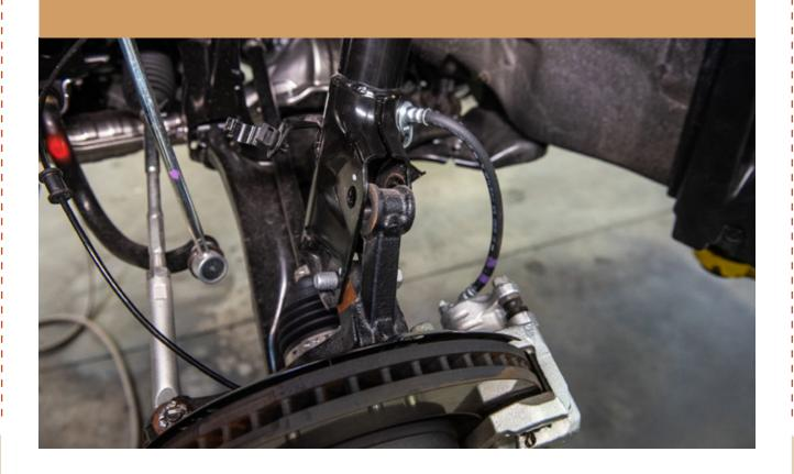
REMOVE THE STRUT ASSEMBLY
