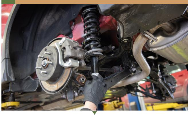
**51** RE INSTALL LOWER BOLTS FOR SHOCKS AND KNUCKLES
