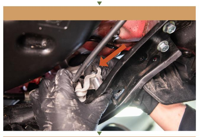
USE A SCREW DRIVER TO KEEP THE BRACKET FROM TURNING WHEN YOU TIGHTEN THE BOLT DOWN.
