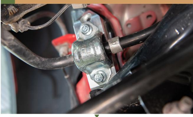
RE INSTALL SWAY BAR MOUNT TO THE VEHICLE
