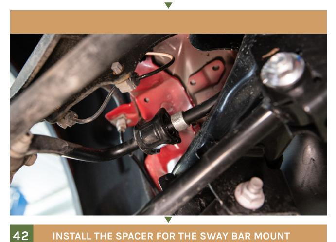
INSTALL THE SPACER FOR THE SWAY BAR MOUNT
