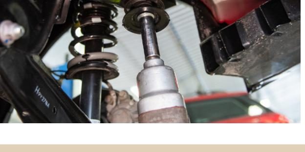
SNUG UP BUT DO NOT TIGHTEN THE BOLTS COMPLETLY
