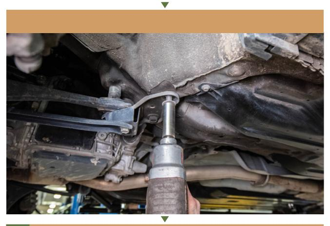
RAISE THE ROCK SLIDER INTO PLACE AND PLACE THE REAR MOUNTING POINT INBETWEEN THE BODY AND THE REAR SUB FRAME BRACKET
