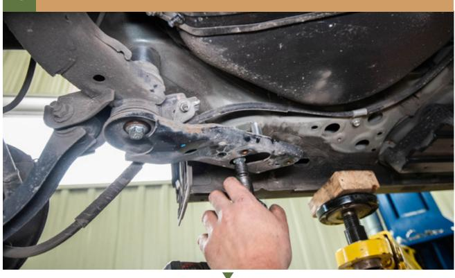
LOOSEN BUT DO NOT REMOVE SUB FRAME BOLT
