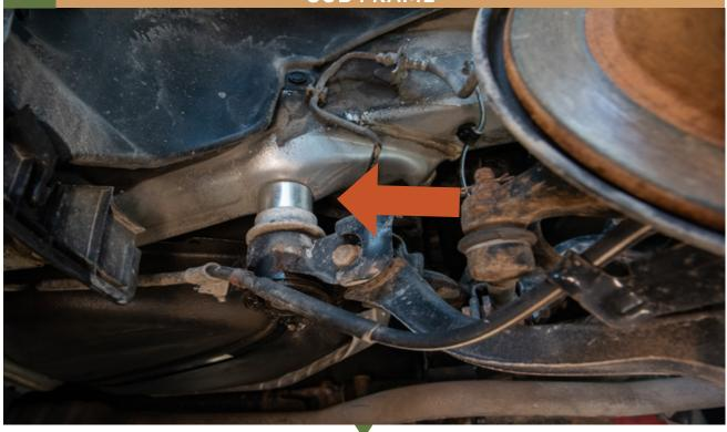
RE INSTALL SUPPLIED SUB FRAME BOLT WITH THE SUB FRAME SUPPORT BRACKET
