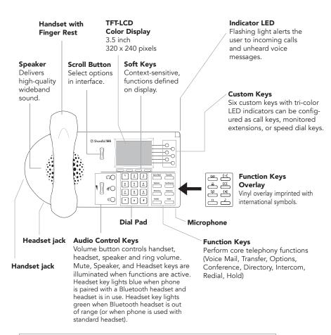
Note: You can connect supported headsets to the 565g IP Phone via the headset jack at the left corner of the phone chassis. Alternatively, you can use this phone with certain Bluetooth-based headset models. Contact your system administrator for details.
