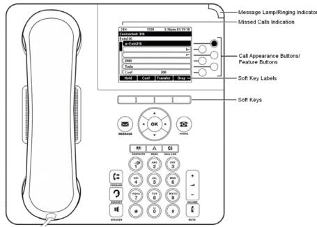
The phone supports 24 programmable call appearance/feature buttons. The labels for 6 of these are displayed in the main display and can be controlled by the adjacent buttons to the right. You can use the  $\triangle$  up/down  $\nabla$  keys to scroll the display. You can also use the  $\triangleleft$  left/right  $\triangleright$  keys to move through the button feature in pages of 6.
