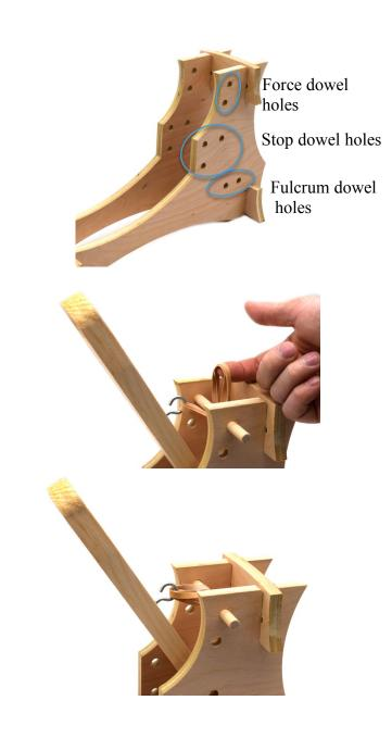
4) Pull back the firing arm and insert the stop dowel. This controls the catapult launch angle. The catapult is now ready to fire.
