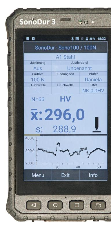
**Motor probes (HV 0,1 – HV 0,8):** 0.1 kgf, 0.3 kgf, 0.8 kgf **Handheld probes (HV 1 – HV 10):** 1 kgf, 3kgf, 5 kgf, 10 kgf
