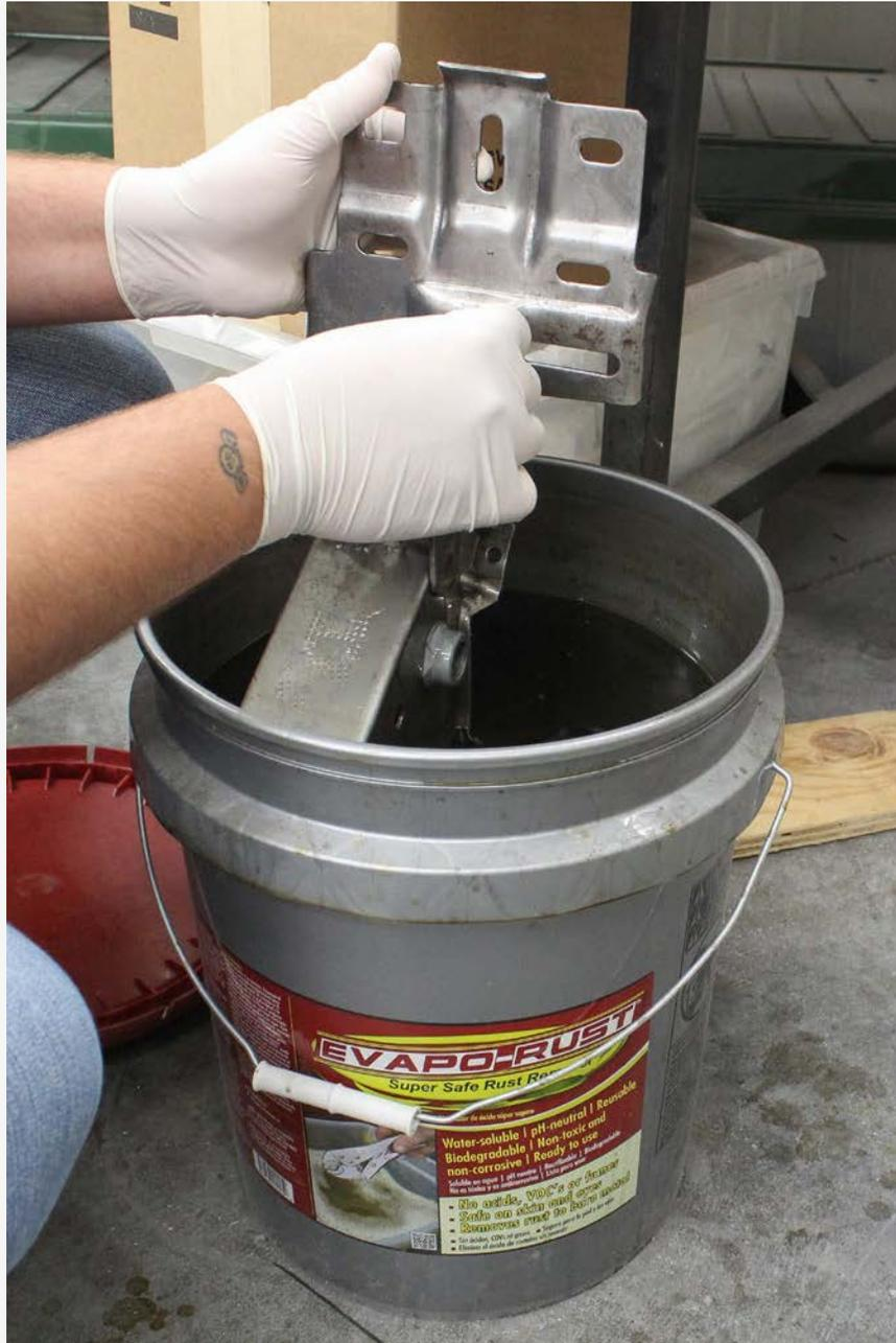
For simple rust like what's on this brake and clutch pedal bracket, MCR relies on soaking the part in Evapo-rust. The product is a liquid that comes in large pails so the parts can be just dropped in and left to soak. Larger parts will require multiple buckets poured into a big plastic bin.
