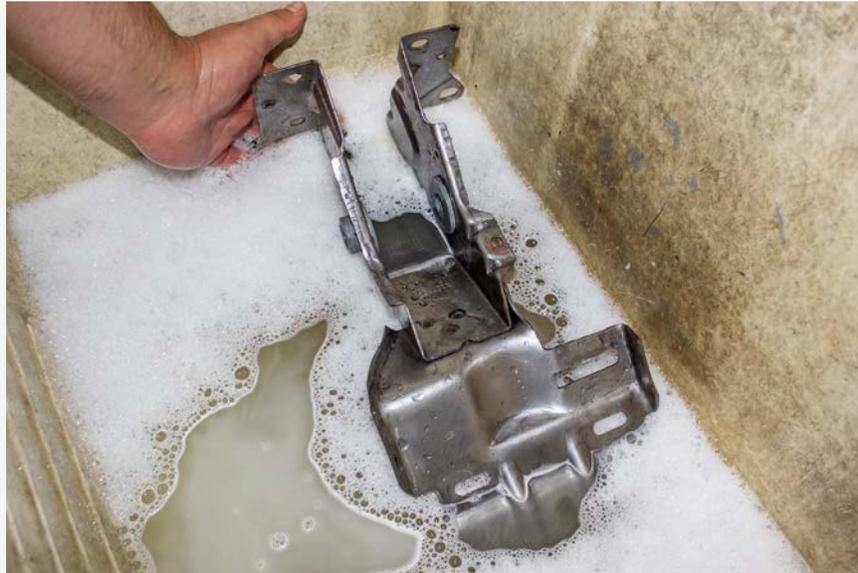
Once the rust is gone, wash the part in hot soapy water to remove the Evapo-rust liquid. Thoroughly dry the part right away to prevent rust from reforming.
