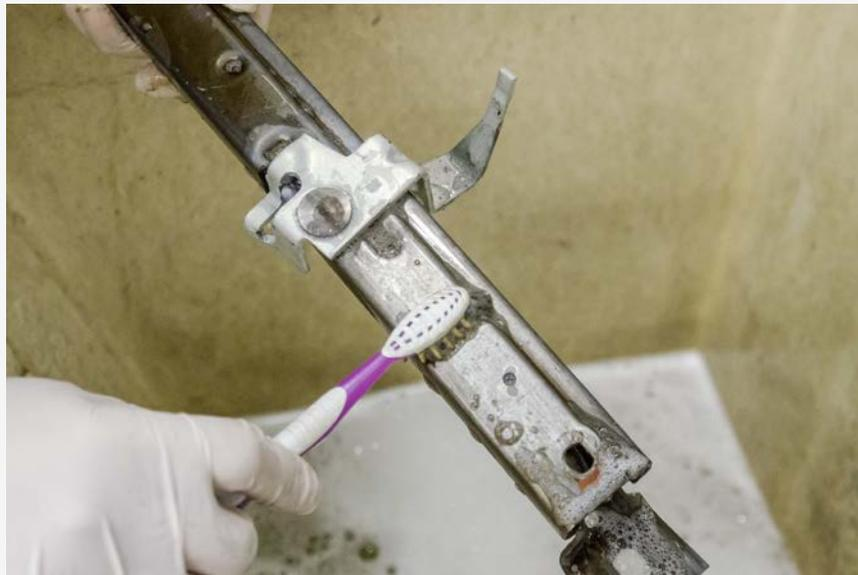
Besides using steel wool to aid in removing rust during the Evapo-rust soak, MCR has found that hot soapy water and a stiff brush can remove the rust and clean the part in one step.
