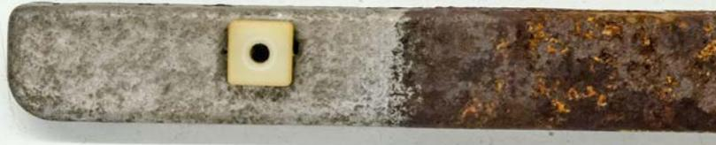
No one would attempt to reuse a part this pitted but it is a great example of how well Evapo-rust will remove rust from even the deepest pits. Notice that it will not harm any plastic parts that may still be attached.
