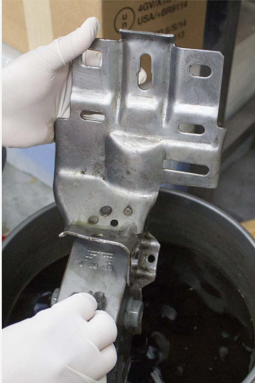
A couple of times a day, lift the part out and gently wipe it with steel wool to remove whatever rust is loose. This will speed the rust removal process. Parts could be clean in a single work day or may need to be soaked for several days.
