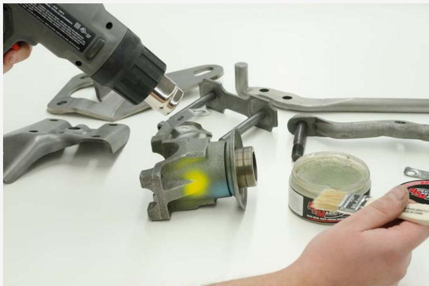
To insure that rust will not return, MCR likes to use a product called Rust Prevention Magic. The part is first warmed with a heat gun or even a hair dryer and then as the paste is applied it liquefies which gives the part a slight gloss which can be seen to help to insure complete coverage. As the part cools, the RPM quickly becomes dry to the touch and looks completely natural and it will not attract dirt. Note that any paint markings will need to be applied before the RPM is used.
