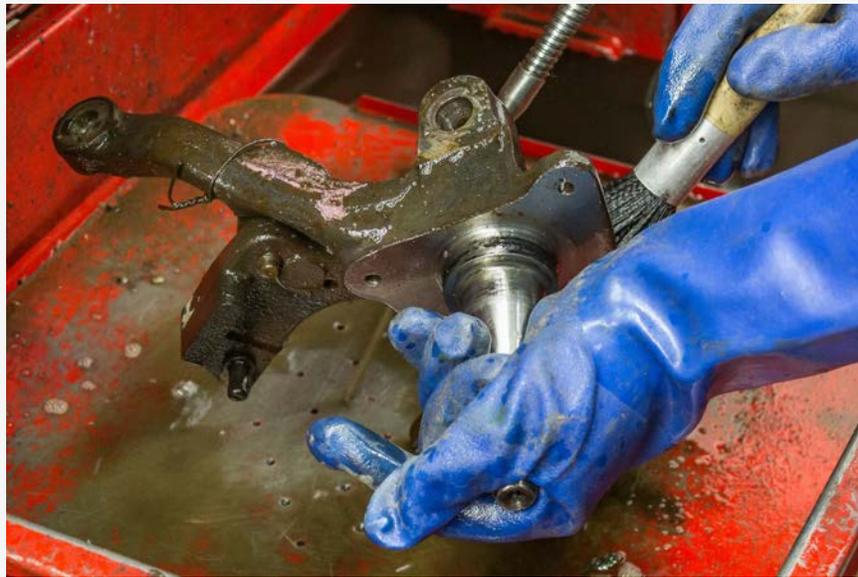
We know this is obvious but for greasy parts the best place to start is the common parts washer and a brush. It does a great job of dissolving away greasy gunk and won't harm any surfaces. For less grimy parts, MCR will use hot water with a good dose of Dawn dishwashing soap and a toothbrush.
