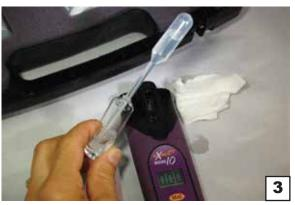
**3.** Take plastic pipette supplied, squeeze bulb with finger and thumb to expel air, and dip pipette tip to the bottom of ampoule and release squeezed bulb slowly to fill pipette (see *Image 3*). Transfer filled pipette liquid to M10 CELL (see *Image 4*).
