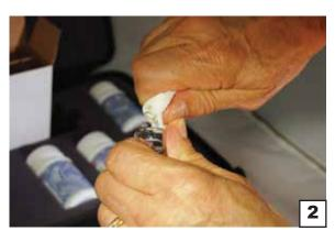
2. Break open one Ready Snap™ 1 Method Verification Solution in a safe manner with a paper towel as shown (see Images 1 and 2).
