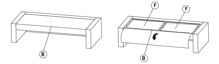
**Step 2--** 1. Turn over Sofa Frame (B), remove the plastic caps on the threaded bolts of each Wood Leg (A). Attach the Wood Legs with Washers (A) x 5 to the corners & the central position of the Sofa Frame (B).
